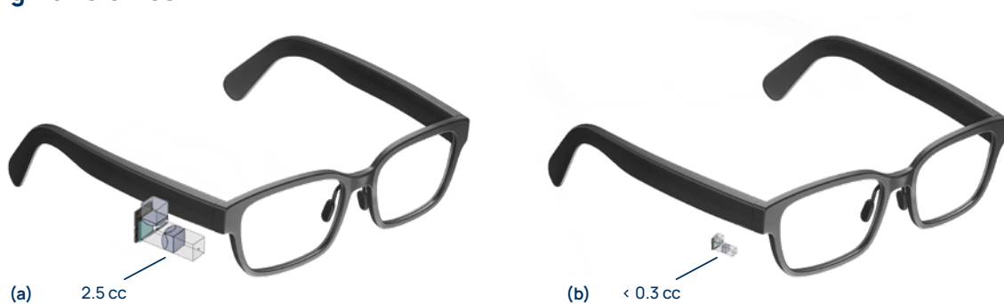
Figure 8: Visualization of foveated 3Kx3K laser-FLCoS engine volumes alongside a glasses frame. (a) Current 7 \mu\text{m} pixel-pitch implementation. (b) Future 2.8 \mu\text{m} pixel-pitch concept. Note, only active optical volumes are shown; mechanical structures are excluded.
