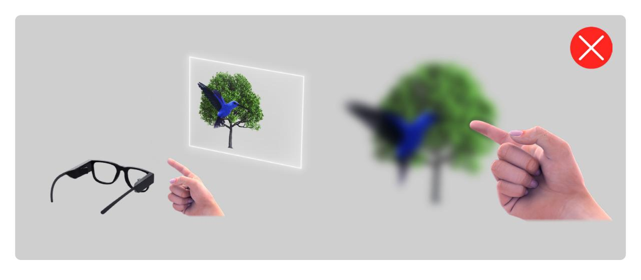
Today's AR displays project a flat image at a fixed focal distance, preventing digital content to blend with the real world.
