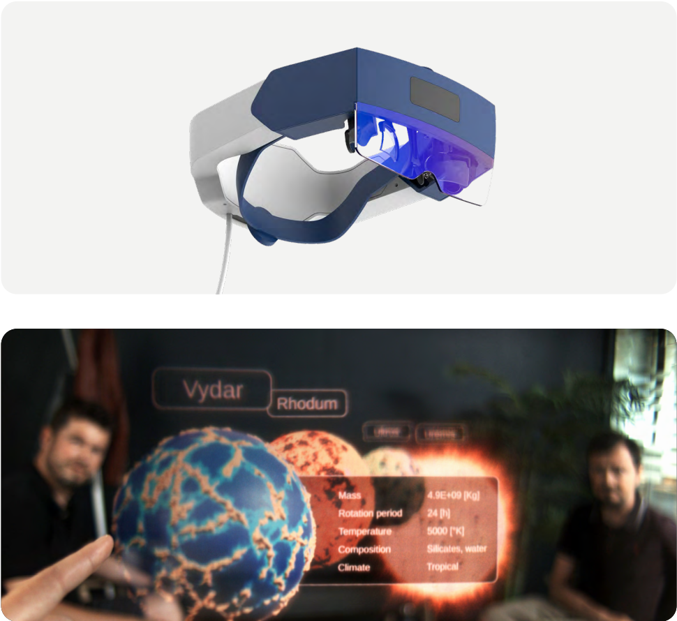
Fig.5: Existing AR digital light field headset and see-through the lens image
