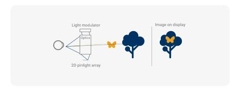
A fast sequence of always-in-focus images passing through a 2D array of viewpoints represents a light field that entirely or almost entirely enters the eye pupil. An eye can then focus on virtual objects in any distance. This operation is performed purely by the eye, no eye-tracking is needed. The light field was already reconstructed and has the properties of the real world light.
