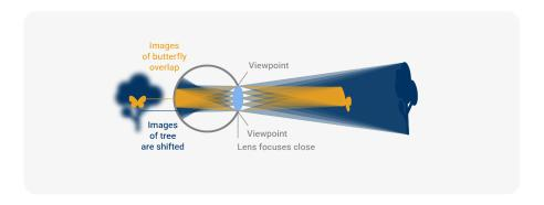
In the CREAL's system, the always-in-focus images are created by a sequential pin-light illumination of a fast spatial light modulator that reflects modulated light beams to imaging optics and towards specific viewpoints in the vicinity of the eye pupil. The modulator is technically a selective mirror that casts a shadow of the scene as it is supposed to be seen from the perspective of the particular viewpoint.
