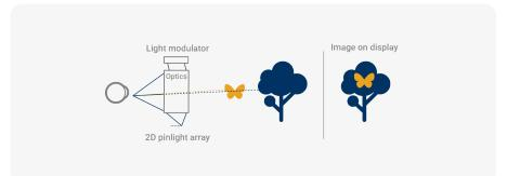
A fast sequence of always-in-focus images passing through a 2D array of viewpoints represents a light field that entirely or almost entirely enters the eye pupil. An eye can then focus on virtual objects in any distance. This operation is performed purely by the eye, no eye-tracking is needed. The light field was already reconstructed and has the properties of the real world light.
