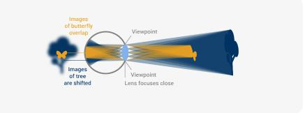
In the CREAL's system, the always-in-focus images are created by a sequential pin-light illumination of a fast spatial light modulator that reflects modulated light beams to imaging optics and towards specific viewpoints in the vicinity of the eye pupil. The modulator is technically a selective mirror that casts a shadow of the scene as it is supposed to be seen from the perspective of the particular viewpoint.
