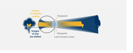
In the CREAL's system, the always-in-focus images are created by a sequential pin-light illumination of a fast spatial light modulator that reflects modulated light beams to imaging optics and towards specific viewpoints in the vicinity of the eye pupil. The modulator is technically a selective mirror that casts a shadow of the scene as it is supposed to be seen from the perspective of the particular viewpoint.
