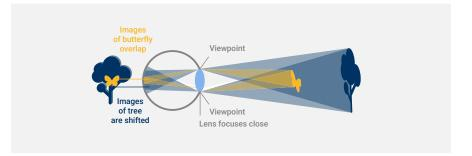
When the eye focuses at the distance of the tree, however, the two images on the retina shift and overlap to create a single sharp image of the tree while the butterfly doubles.
