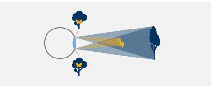
The eye lens then controls the mutual position of the images. If the eye focuses at the distance of the butterfly, the two images of the butterfly, each projected through a different viewpoint, overlap to create its sharp image, while the objects in another distances, such as the far tree, appear mutually displaced.
