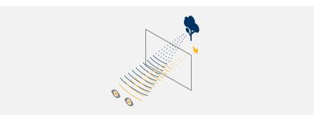
Light field is a practical and simple approximation of real world light. Instead of treating light in terms of waves like CGH, it treats light in terms of rays or photons that bombard the eye from virtual points in space and build their image on the retina. Most of the realizations so far, however, provided low quality imagery. The rest of the document will be therefore about light fields, their current deficiencies, and how to make light fields work efficiently, well and now.
