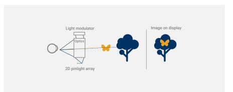
A fast sequence of always-in-focus images passing through a 2D array of viewpoints represents a light field that entirely or almost entirely enters the eye pupil. An eye can then focus on virtual objects in any distance. This operation is performed purely by the eye, no eye-tracking is needed. The light field was already reconstructed and has the properties of the real world light.
