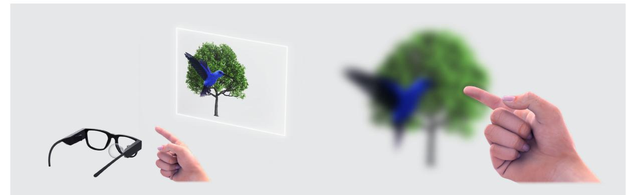
Today, most AR glasses display flat images at a **fixed focal distance** ... ... preventing our eyes to focus correctly on objects at another distance.
