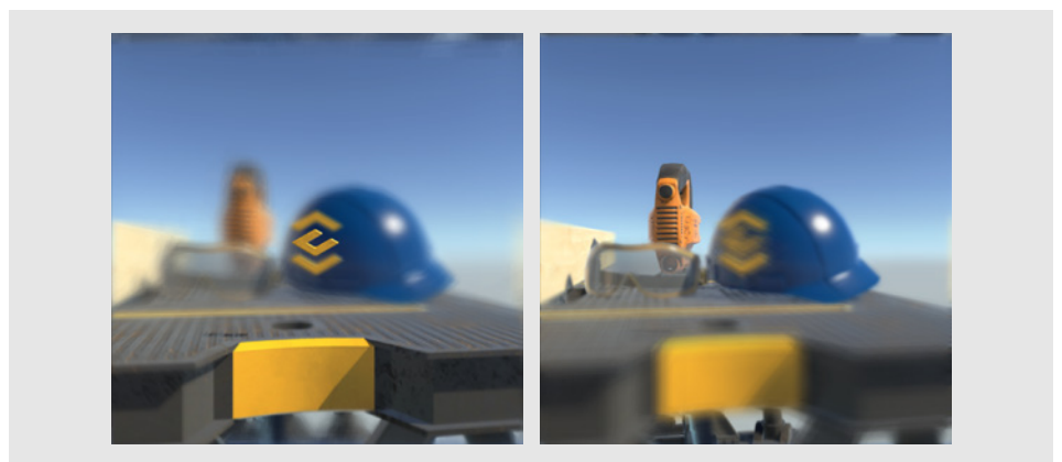
Simulation of the focus on two different distances, obtained by averaging the views that form the pupil. One can see that it yields convincing bokeh although individual views are not perfect. Left is focused on the close logo and right on the farther jigsaw.
