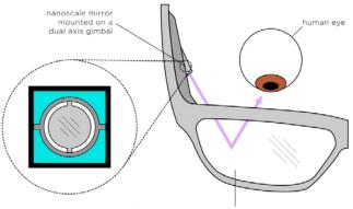
holographic combiner: holographically embedded mirror-like elements, within a prescription lens
